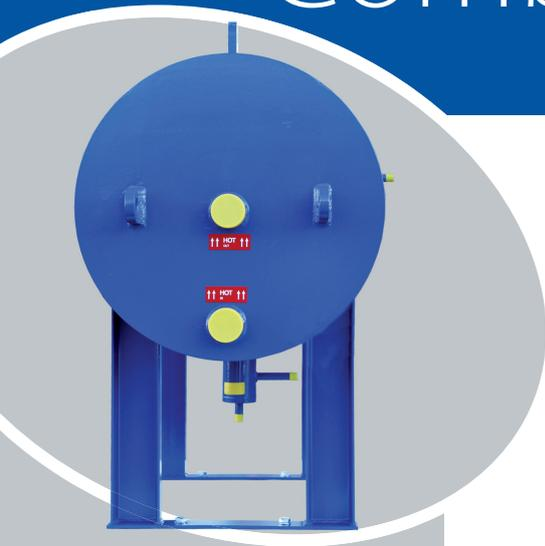
**V**ahterus Combined is a compact solution available for use with both flooded evaporators and flooded cascades. These Combined solutions integrate the evaporator and separation system within a single vessel, creating a compact solution with low refrigerant charge.
