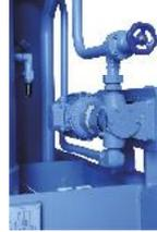
Pre-lubrication oil pump, for booster with permanent pump
