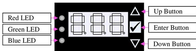
The user interface is located on the front of the valve and when in normal operation will display the % open of the valve Vport. The setup menu can be entered to automatically calibrate, adjust the control parameters, and view current settings. All displays in this menu start with the letter “H.”. The keypad and display are shown below.
